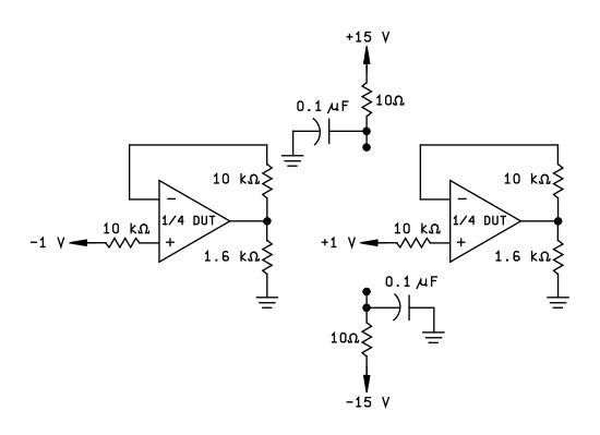
FIGURE 2. Radiation exposure circuit.
